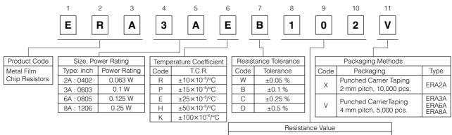
Consist of three figures for E24 series resistance value. The first two digits are significant figures of resistance and the third one denotes number of zeros following. (example) 102 : 1 k $\Omega$
